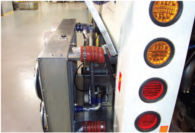
All of the new cooling system components were mounted on a sliding tray to facilitate service and maintenance access.
