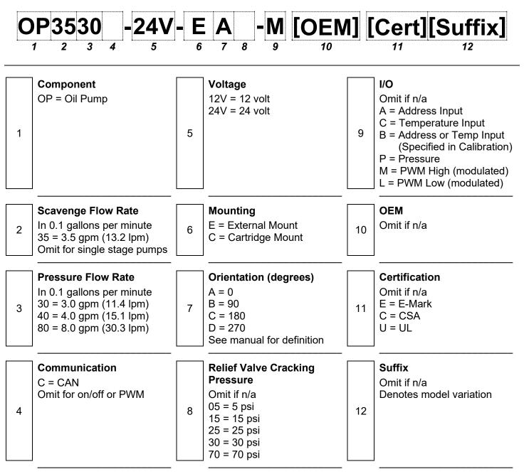
**OP3530-24V-EA-M** = Oil Pump. 3.5 gpm scavenge/3.0 gpm pressure, on/off/PWM communication, 24 Volt External Mount at 0 degrees, no relief valve, uses PWM High input for commands.
